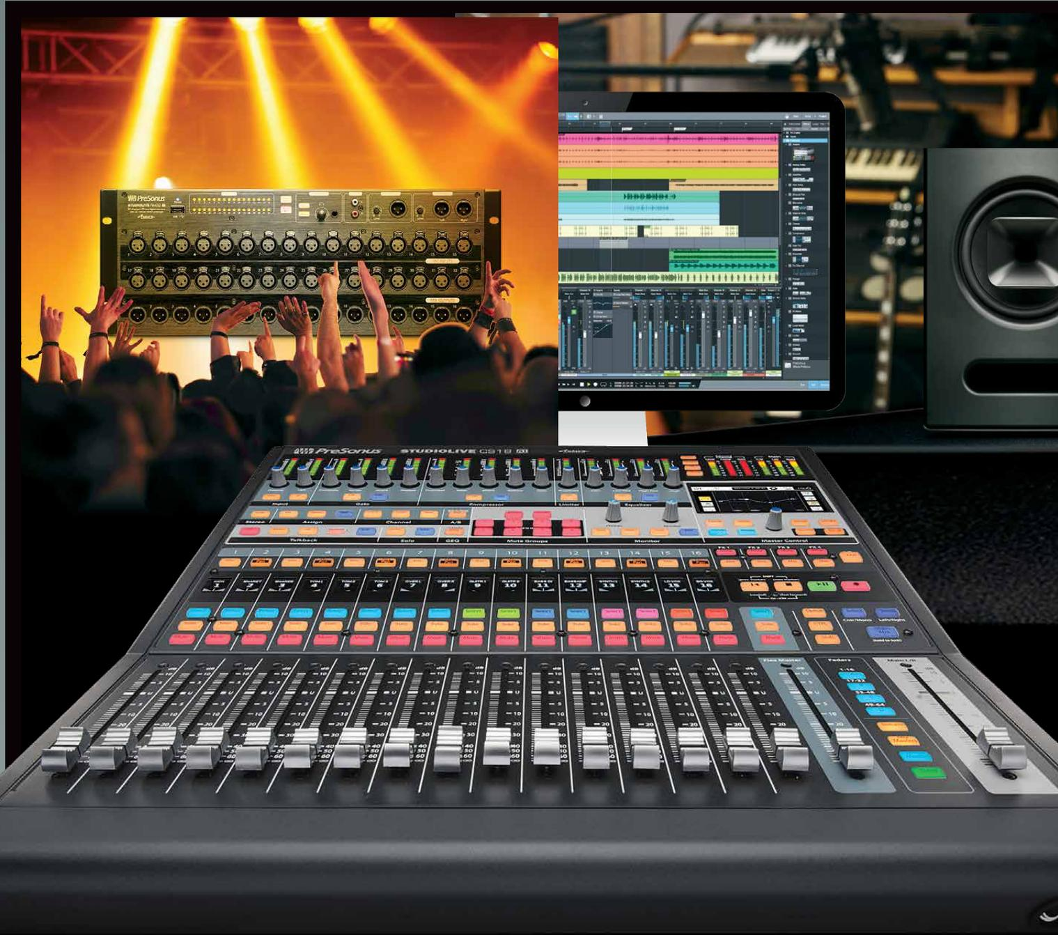
Using AVB networking for control and audio transport, CS18AI users can remotely operate RM mixers and take advantage of local 4x2 audio IO
